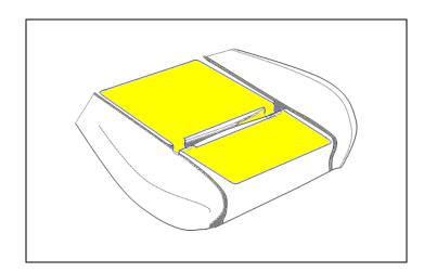
3) The listing channels or the Velcro hold-downs should line up with the cutouts in the heating elements. Seat heater adheres 100% to the foam bun following the surface into the listing gaps. Opening in heater is aligned with gap.
