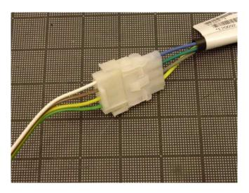
1) This is the 4 Pin connector at the end of the element harness. Disconnect the bonded wire harness and use a multi-meter to check for continuity.
