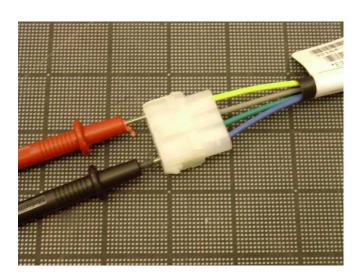
2) Set the multi-meter to ohms, and touch the red and black probes to the yellow and blue pins. The meter should show That there is continuity through the heating wire; if it does not, there is a break in the heating wire.
