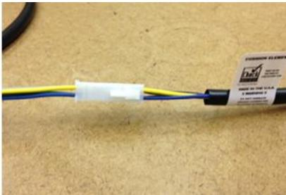
1) This is the 4 Pin connector at the end of the element harness. Disconnect the wire harness and use a multi-meter to check for continuity.
