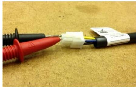
2) Set the multi-meter to ohms, and touch the red and black probes to the yellow and blue pins. The meter should show that there is continuity through the heating wire; if it does not, there is a break in the heating wire.
