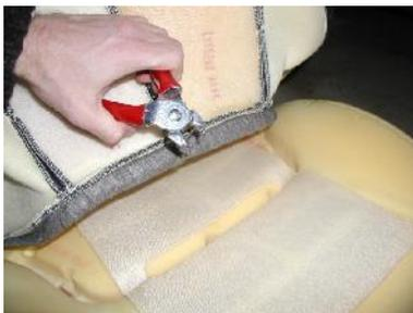
3) The listing channels or the Velcro hold-downs should line up with the cutouts in the heating elements. Seat heater adheres 100% to the foam bun following the surface into the listing gaps. Opening in heater is aligned with gap.
