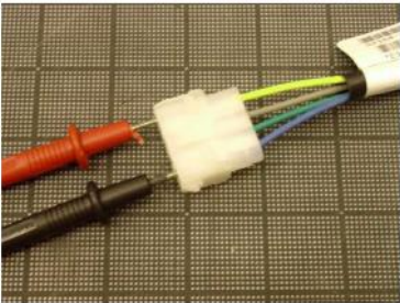
Figure 2: Set the multi-meter to ohms, and touch the red and black probes to the yellow and blue pins. The meter should show that there is continuity through the heating wire. If it does not, there is a break in the heating wire.
